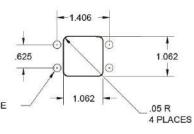
BOTTOM MOUNT-CLEARANCE HOLE FOR .192 SCREW TOP MOUNT-CLEARANCE HOLE FOR .112 SCREW
